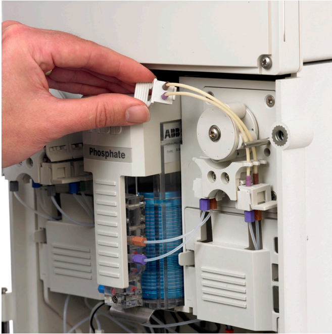
Figure 4 Simple to replace pump tube assemblies
