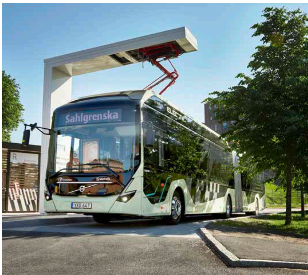
A brief top-up at the bus station: Volvo bus and ABB charging infrastructure.
