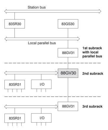
The 88GV30 module shall be installed only on the far right on a subrack.
