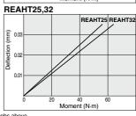
Note) Deflection when a moment other than the above is applied can be specified by extending the lines in the graphs above.
