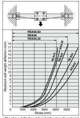
The above deflection data indicate values for external movement within the stroke.
