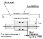
Note)Referring to the self-weight deflection in the graph below, provide clearance so that the cylinder does not touch the mounting surface or the load section, and is able to operate smoothly within the minimum operating pressure range for a full stroke.
