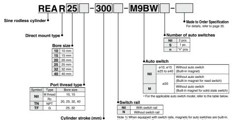
Note 2) In the case of ø15, magnets for auto switches are built-in even when not equipped with switch rails
